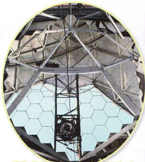
The mirrors on The Hobby-Eberly Telescope at the McDonald Observatory, Texas, America.
