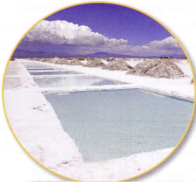
Salt works are used to extract salts from seawater using evaporation.
