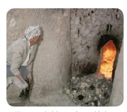
▲ Limestone (calcium carbonate) being heated in a lime kiln to give calcium oxide (called lime, or quicklime). The lime might be used to make limewash for buildings, or mixed with sand to make lime mortar.
