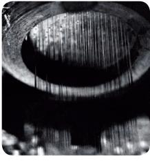
A Fibres of nylon and Terylene are made by pumping the melted polymer through a spinneret (like a shower head). As it comes out through the holes, the polymer hardens into long threads.
