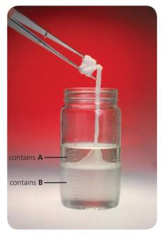
▲ Making nylon in the school lab. **A** is dissolved in water. **B** is dissolved in an organic solvent that does not mix with water. Nylon forms where the solutions meet.
