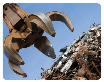
▲ Very often, scrap iron is added to the molten pig iron in the oxygen furnace. So the iron gets recycled as new steel.
