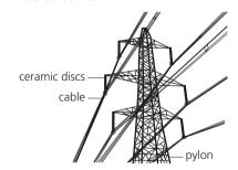
At pylons, ceramic discs support the bare cables. Since it is an insulator, the ceramic prevents the current from running down the pylon. (Dangerous!)
