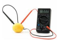
▲ The conductivity meter measures the current passing through the liquid, carried by ions. (Lemon juice contains hydrogen ions and citrate ions.)
