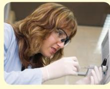
▲ Injecting a sample into the carrier gas, at the start of gas chromatography.
