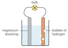
At the same time bubbles of hydrogen start to form on the copper strip, and the magnesium strip begins dissolving.
