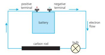
The photograph above shows a battery, a bulb and a rod of graphite joined or **connected** to each other by copper wires. (Graphite is a form of carbon.) This arrangement is called an **electric circuit**.
