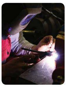
▲ Welding is often carried out in an atmosphere of argon, which will not react with hot metals (unlike oxygen).
