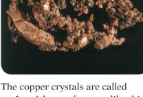
**grains**. A lump of copper like this one consists of millions of grains joined together. You need a microscope to see them.
