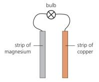
Connect a strip of magnesium, a strip of copper, and a light bulb, like this. (Note: no battery!) Nothing happens.
