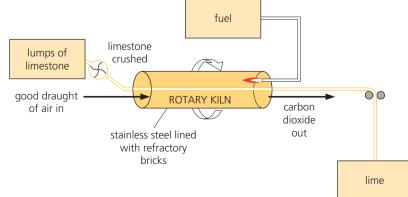
A rotary kiln for making lime.
