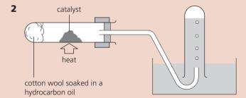
A hydrocarbon can be cracked in the lab using the apparatus above.
