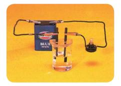
**Ethanol.** The liquid is connected into the circuit by placing graphite rods in it. The bulb does not light, so ethanol is a non-conductor.
