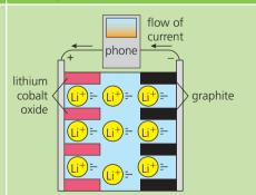
When you use it, the lithium ions flow back to lithium cobalt oxide, and electrons flow from the graphite to power your phone.
