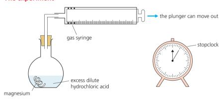
Clean the magnesium with sandpaper. Put dilute hydrochloric acid in the flask. Drop the magnesium into the flask, and insert the stopper and syringe immediately. Start the clock at the same time.
