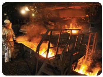
▲ Iron occurs naturally in the earth as iron(III) oxide, Fe<sub>2</sub>O<sub>3</sub>. This is **reduced** to iron in the blast furnace. Here, molten iron runs out from the bottom of the furnace.
