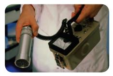
▲ Checking for radiation using a Geiger counter. The meter gives a reading, and you may also hear beeps.
