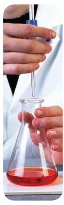
▲ The colour of the solution has changed: the titration is complete.
