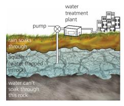
▲ Using an aquifer as a water supply.
