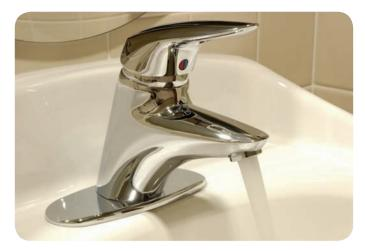
A steel tap plated with chromium, to make it look bright and shiny. Chromium does not stick well to steel. So the steel is first electroplated with copper or nickel, and then chromium.
