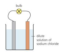
Now stand the strips in a dilute solution of sodium chloride. Something amazing happens: the bulb lights! A current is flowing.
