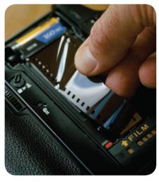
▲ Putting film in a camera. Most of the film is inside the yellow cartridge, at the top, protected from light.
