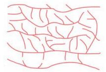
At about 200 °C, 2000 atmospheres pressure, and with a little oxygen present, the chains will branch. Now they can't pack closely, so the polythene is far less dense.
