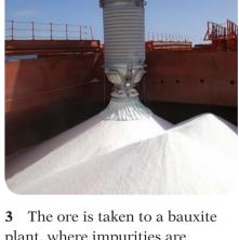
**3** The ore is taken to a bauxite plant, where impurities are removed. The result is white **aluminium oxide**, or **alumina**.
