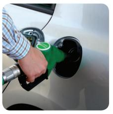
This petrol pump can pump out petrol at a **rate** of 50 litres per minute.
