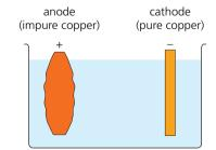
The anode is made of impure copper. The cathode is pure copper. The electrolyte is dilute copper(II) sulfate solution.
