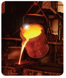
▲ Molten iron being poured out at an iron works. Hot – over 1540°C!
