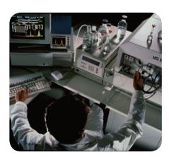
▲ A mass spectrometer, for finding relative molecular mass. It compares the mass of a molecule with the mass of a carbon-12 atom, using an electric field.
