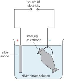
▲ Silverplating: electroplating with silver. When the electrodes are connected to a power source, electroplating begins.
