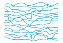
At about 50 °C, 3 or 4 atmospheres pressure, and using a catalyst, you get long chains like these. They are packed close together so the polythene is quite **dense**.
