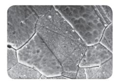
The regular arrangement of ions results in **crystals** of copper. This shows the crystals in a piece of copper, magnified 1000 times. (They are all at different angles.)
